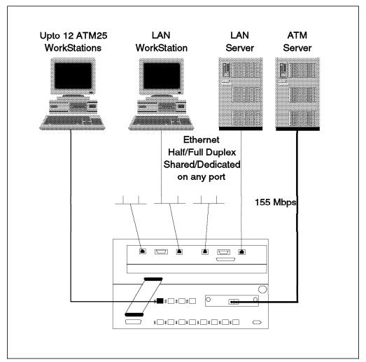
Figure 24. Local LAN Bridging and ATM Server Access
